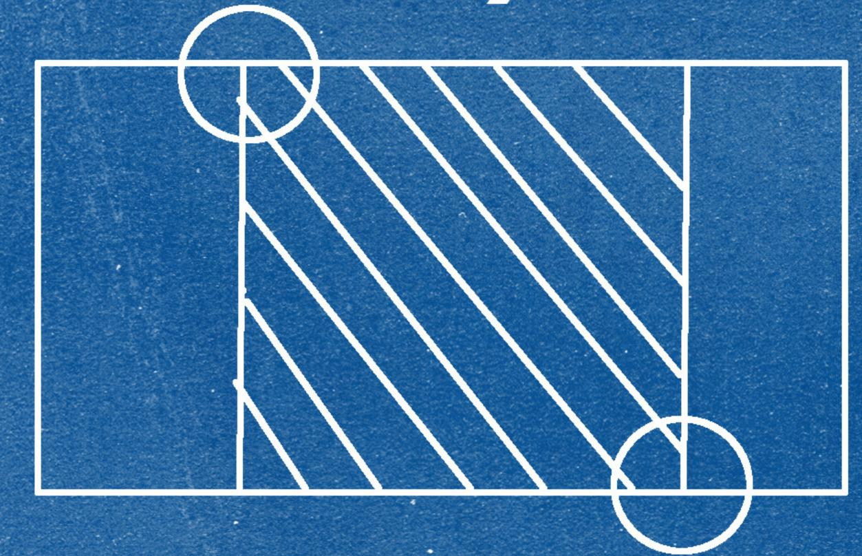
Lay out a square on the end of your stock. Connect two corners and you'll have an instant 45 degree bed. Use those corners to carry your layout lines across the top and bottom of your stock. These lines will give you the top and bottom edges of the bed.
